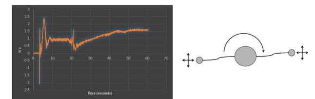
In the event of a pressure source malfunction where the correct internal pressure could not be reached, the concept spacecraft could still generate artificial gravity. If there was an adequate supply of reserve propellant to correct for deviations in trajectory due to the increased duration of instability before the 1g equilibrium is reached, the inflatable beams act as a tether. This result is not surprising, but perhaps overlooked during the experiment planning.
