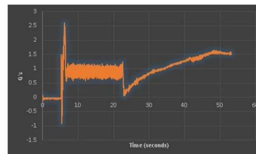
For the brief instant during spin-up, the .02 pound inflatable resisted buckling against an equivalent force of .92 pounds during the maximum impulse. Resisting buckling against 42 times the inflatable's own mass is quite impressive.
